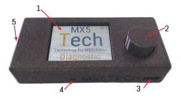
1=Display Screen 2=Control knob. Turn and press. 3=USB Socket. 4=Sounder 5=Connection Pins (Underneath)
